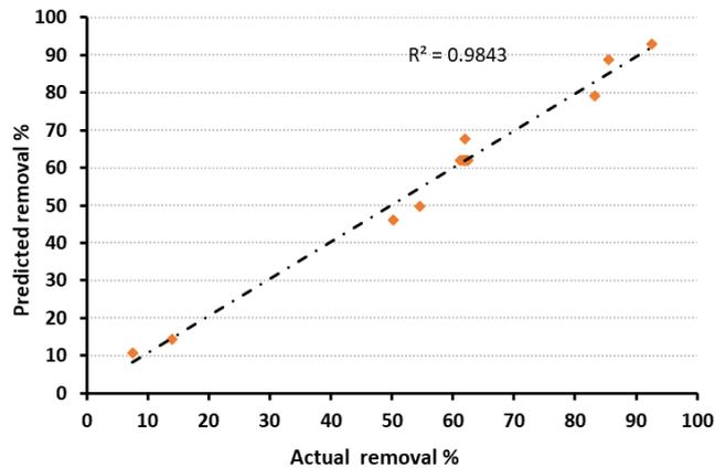
**Figure 2.** Predicted Vs experimental nitrate removal.
