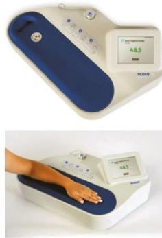
Figure 1. Photographs of the SCOUT DS skin fluorescence spectrometer. The fluorescence of the left volar forearm skin is noninvasively measured by the fibre optic array visible in the top left (Vlahoman et al., 2020).
